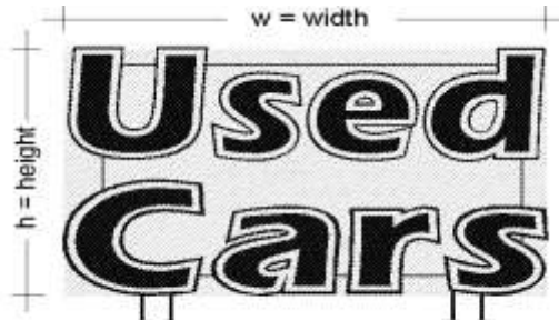
Calculating Area of a Sign where Copy Exceeds Sign Area = (height of copy) x (width of copy)
